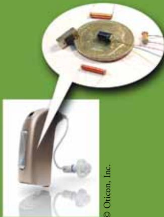
The telecoil, a small copper wire, is located inside the hearing aid.
