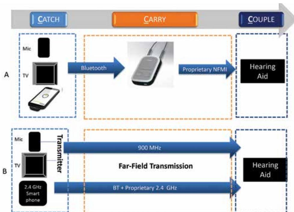
**Figure 1A and B. Principle behind wireless connectivity: The sound is captured, carried and coupled to the listener.**
